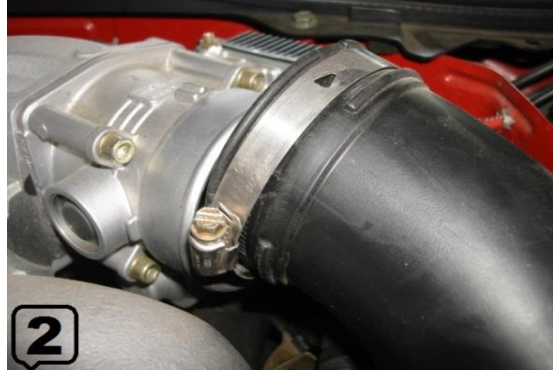
2. Remove the Clamp on Throttle Body
