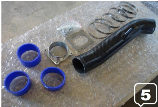
5. This is Over View of Carbon Fiber Intake Kit (Air Filter is Not Show / use any brand 3" Inlet Air Filter with this Intake Kit)
