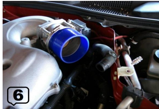
5. This is Over View of Carbon Fiber Intake Kit (Air Filter is Not Show / use any brand 3" Inlet Air Filter with this Intake Kit)
