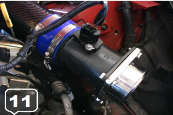
11. Mount the Stock MAF Sensor back on the Stock MAF Sensor Tube and Install the Aluminum MAF Adapter the Stock Tube using the 4 bolts as illustrated above step
