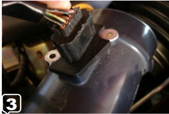
3. Remove the 2 Bolts on MAF Sensor
