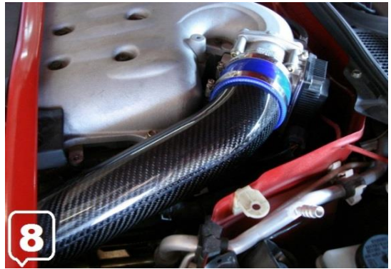
8. Than Mount the Carbon Fiber Intake Pipe to the Silicone Hose to the Throttle Body Side
