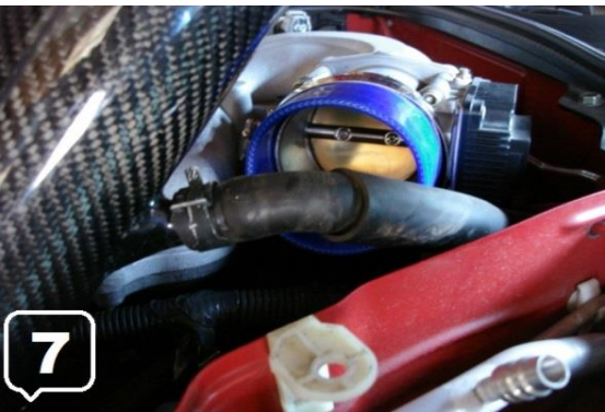
7. Connect the Stock Lower Vacuum Hose to the New Carbon Fiber Intake Pipe at Lower section
