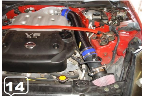
14. Front View of Installed Carbon Fiber Intake Kit
