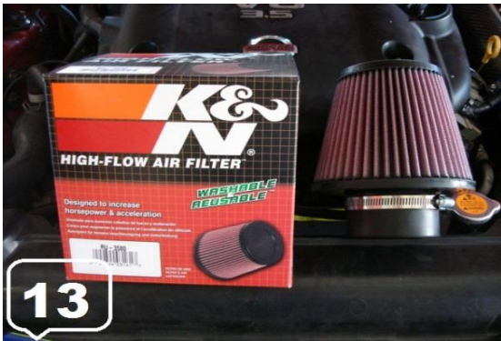
13. Then you can use any Brand Open Element Air Filter with this Carbon Fiber Intake Kit (Air Filter must be in 3" Inlet) We used K&N 3" Filter for this Kit
