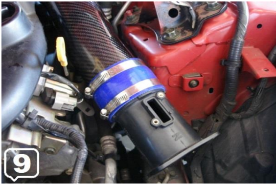
9. Mount the Stock MAF Sensor Tube with 3" Silicone Hose with 2 Clamps
