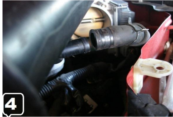
4. Remove the Lower Vacuum Hose
