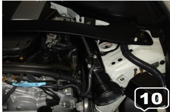
10. Overview of Driver Side Carbon Fiber Intake Installed with MAF Sensor back on the Pipe.
