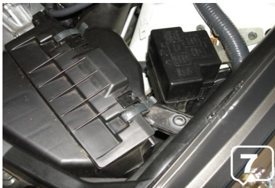
7. Remove the 10mm Bolt x 1 Holding the Stock Air Box / and Pull straight out
