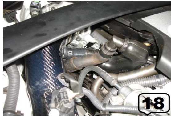
18. Vacuum Hose connected to the Carbon Fiber Intake Vacuum Tube / due to lack of mounting space you need to tilt the stock Vacuum Resonator Upward like shown in picture
