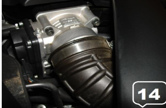
14. Remove the Clamp on Passenger Side Throttle Body / Remove the Stock MAF Sensor Holding by 2 Screws
