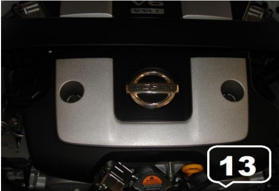
13. Before Start on Passenger Side Stock Intake Removal / Need to Remove this Plastic Cover with 10mm socket tools x 2 bolt
