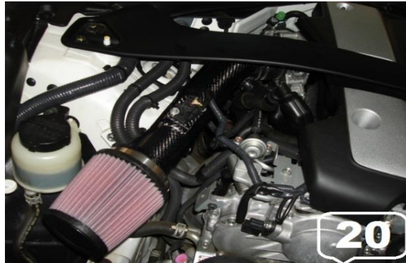
20. Overall view on Passenger side Carbon Fiber Intake Installed with MAF Sensor and K&N Air Filter back on the Intake Pipe
