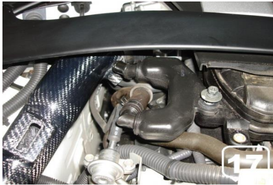
17. Loosen up the Bolt 10mm x 1 Holding the Vacuum Resonator for Easy access on Connecting the Vacuum Hose on the Carbon Fiber Intake Vacuum Tube
