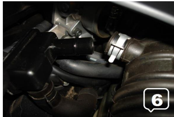
6. Remove the Vacuum Resonator off the Stock Intake Hose
