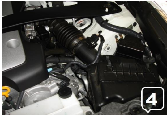
4. Driver side Stock Intake System / Remove the Stock MAF Sensor Holding by 2 Screws
