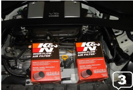
3. You can use any brand Open Element Air Filters x 2 pcs with this Carbon Fiber Intake kit (Air Filter must be in 3.5" Inlet) We used K&N 3.5" Filter for this Kit
