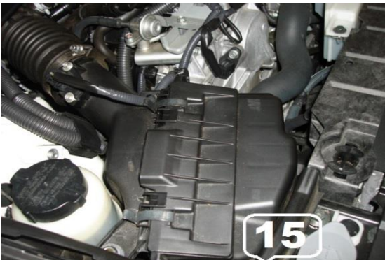
15. Remove the 10mm Bolt x 1 Holding the Stock Air Box / and Pull straight out
