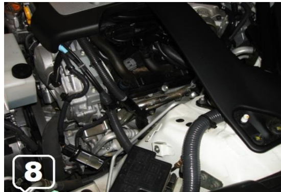
8. This is the Empty Driver side space with Stock Air Intake System Removed
