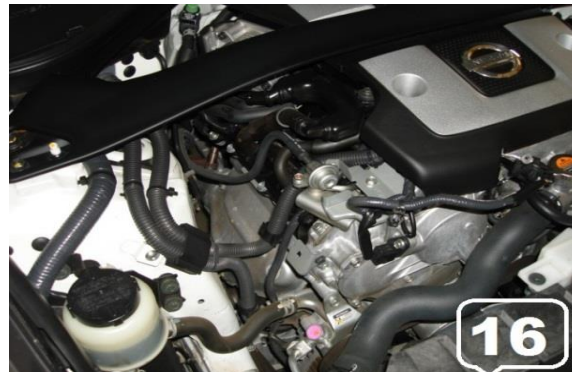
16. This is the Empty Passenger side space with Stock Air Intake System Removed
