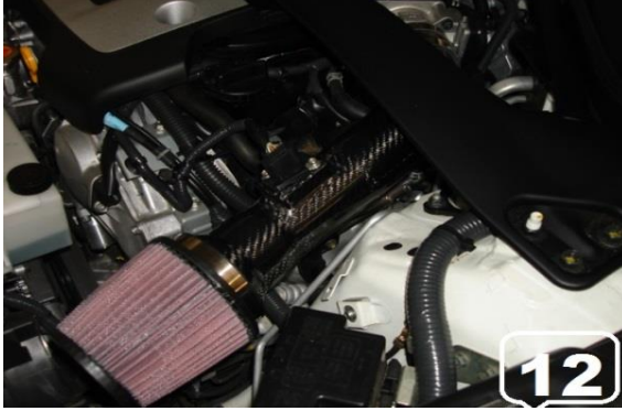
12. Driver Side Carbon Fiber Intake with K&N Air Filter Installed / Driver Side Installation Completed
