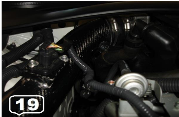
19. Mount the Stock MAF Sensor back on the Carbon Fiber Intake Pipe
