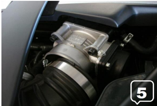
5. Remove the Clamp on Driver Side Throttle Body
