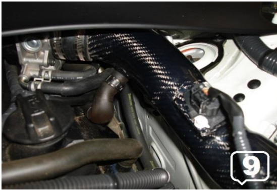
9. Mount the Driver Side Carbon Fiber Intake Pipe to Throttle Body and Mount the Vacuum Hose back on the Tube with Stock MAF Sensor back on the Pipe
