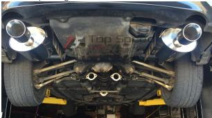
Locate the secondary pipe with the Top Speed Tag, this goes on the passenger side between the muffler and mid-pipe. Add gasket and hand tighten bolts on.
