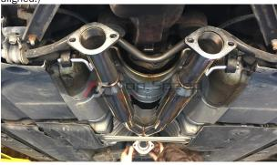
7. Attach the Top Speed Mufflers to the 2 hangers on the driver and passenger side.
