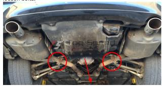
3. Disconnect the 2 hangers (one on each side) from the mid-pipe. After, pull and remove the mid-pipe out.
