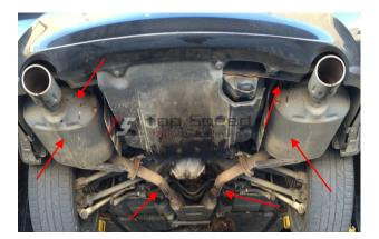
Remove 2 bolts between the mid-pipe & y-pipe, and 4
